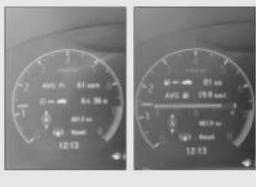
Driving 400 km, all on highways and using cruise control, the City CVT returned fuel efficiency of 19.9 km/litre (more than the claimed 18.4 km/litre). We set cruise control at 85 km/h for this trip, and the average speed recorded was 61 km/h.
